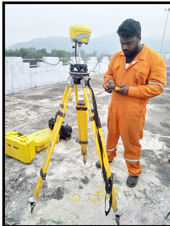
Figure 5.3-1 DGPS Observation at Dam top
